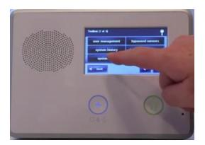
2. Once the panel is in a system test, you can open the individual sensor and replace the batteries.
