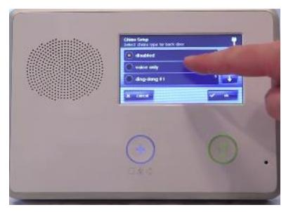
5. After chimes have been created, you will need to enable the chime feature. To do this, press **Security**, **Menu**, and check mark the chime button on the bottom of the touch screen.
